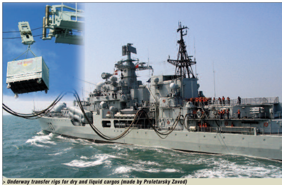
> Underway transfer rigs for dry and liquid cargos (made by Proletarsky Zavod)
